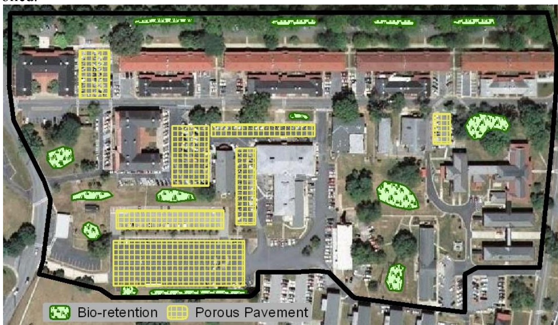
Figure 18. Actual Site and Onsite Control Measures (Atlanta, GA)
